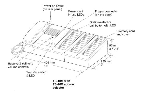
The selector switch bank is aligned vertically, with each station having its own directory. Station numbers count top to bottom 1 to 10 on first switch bank, and 11 to 20 on the second switch bank of TB-20M. The supplied directory card and cover can be attached from the left.
